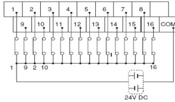
Figure FCJ Digital Input Terminal Numbers and External Connections
