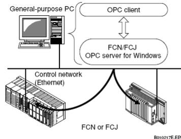
Figure Example of the System: FCN/FCJ Autonomous Controllers operate linking with OPC Servers for Windows
