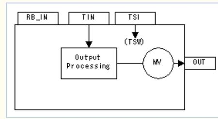
FIGURE: Block diagram of the Manual Loader POU
