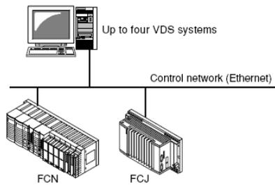
Figure A System where FCN/FCJ Autonomous Controllers Operate by Linking with a VDS System
